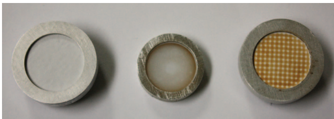
FIG. 4. Particle deposition patterns on a conventional passive sampler, a single-domain MPAS, and a multidomain MPAS (from left to right), which were exposed simultaneously inside the RAWT.
